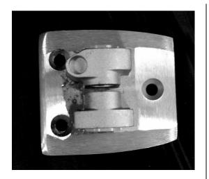
2. Set and push spring with slight pressure into spring pocket.
