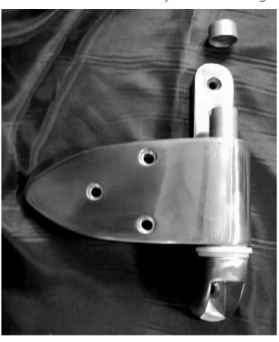
2. Turn hinge upside down with back of hinge facing you. Rest base on protected surface. Using rubber tipped hammer forcefully strike side of hinge blade close to the base.
