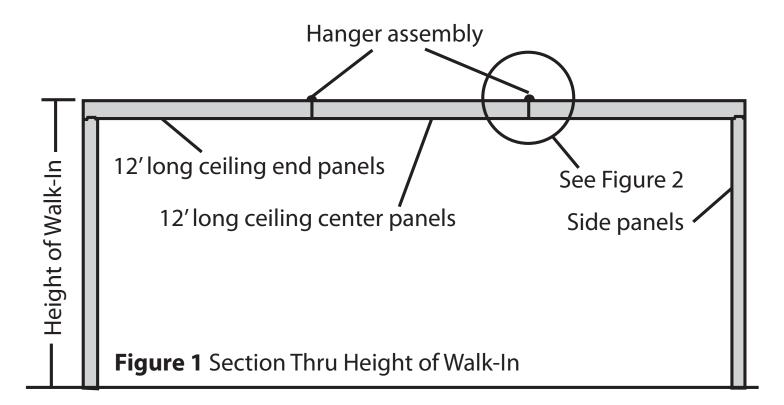
Note: It is important NEVER to walk on top of a Bally ceiling that is not supported by interior steel or other temporary structural supports. Failure to support ceiling will cause joint failure and likely cause serious injury or death.
