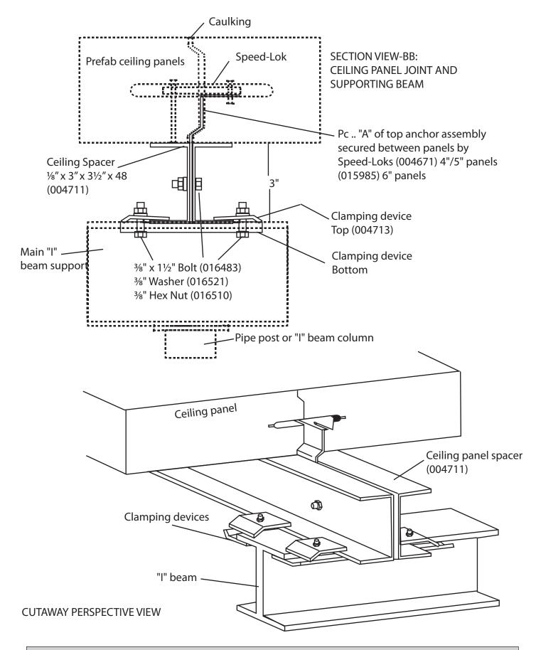
Note: It is important NEVER to walk on top of a Bally ceiling that is not supported by interior steel or other temporary structural supports. Failure to support ceiling will cause joint failure and likely cause serious injury or death.
