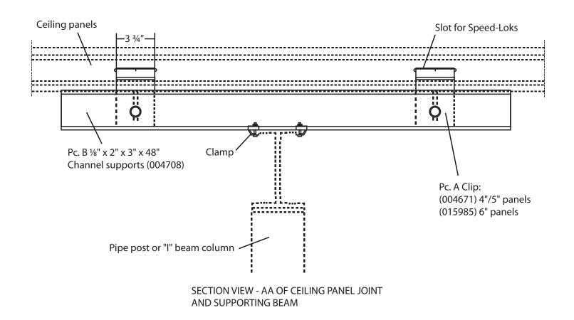
Note: It is important NEVER to walk on top of a Bally ceiling that is not supported by interior steel or other temporary structural supports. Failure to support ceiling will cause joint failure and likely cause serious injury or death.
