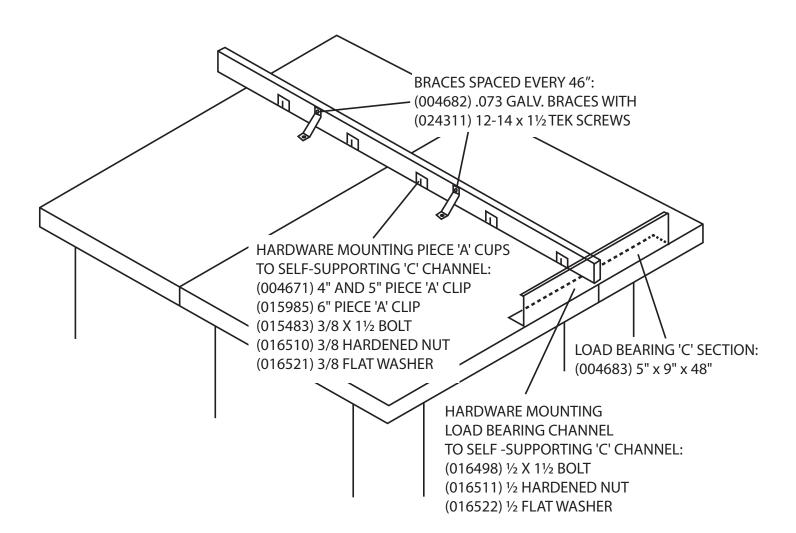
Note: It is important NEVER to walk on top of a Bally ceiling that is not supported by interior steel or other temporary structural supports. Failure to support ceiling will cause joint failure and likely cause serious injury or death.
