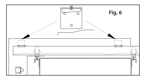
The **Padlock Bar** is clamped onto the frame with the emergency release handle.
