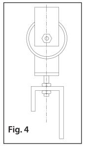
Figure 4: Install the Roller Brackets into the aluminum brackets screwed to the upper sides of the door cap, capturing the bracket between the two nuts. The upper nut is most likely where it was when we took the door down, so try not to adjust it. Leave the lower nut down somewhat, you want the brackets loose at this point.
