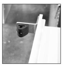
The **Floor Roller** keeps the door from swinging away from the wall, and presses the gasket against the wall when the door is closed. Position the base as shown (*Fig. 7*) and bolt to the floor. The angled plate in the sketch is already attached to the door.
