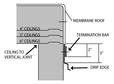
NOTE: THE DRIP EDGE SHOULD BE INSTALLED BEFORE ATTACHING THE DOWNWARD EDGE OF THE MEMBRANE ROOF. ALIGN THE TOP OF THE DRIP EDGE WITH THE CEILING TO VERTICAL JOINT. ATTACH DRIP EDGE AT TWO OR THREE LOCATIONS TO TEMPORARILY HOLD IT IN PLACE. NOW COMPLETE INSTALLATION OF MEMBRANE ROOF.
