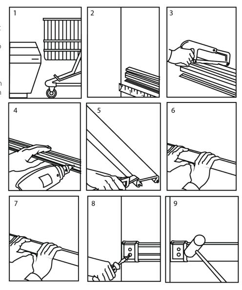
9. Hammer end/corner cap on edge to seat teeth into vinyl. Tighten screws. Insert plugs to conceal screws.
