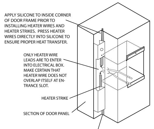
RUN HEATER ELEMENT TO BOTTOM OF DOOR FRAME AND MAKE LOOP AT THE BOTTOM. (SHOWN WITHOUT SILICONE).
