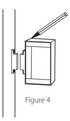
Position the T-11 box, with the switch temporarily mounted, and match it up to the magnet with the door fully closed. The switch has a 1" actuation range, so feel free to leave a gap around 1/2". Mark the location and drill mounting holes. (Fig. 4)
