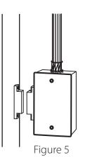
Install the box and conduit. Pull the cable, strip and attach the leads to the connections while the switch is still loose, then install the switch and cover. (Fig. 5)
