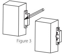
On the T-11 box, flush the front side of the switch with the top of the box, and mark the mounting hole centers & back edge onto the box. Drill 1/8" for the mounts & a 5/816" hole at the middle of the line. The large hole will make it easier to wire the switch and yet will be entirely beneath the switch & cover. (Fig. 3)
