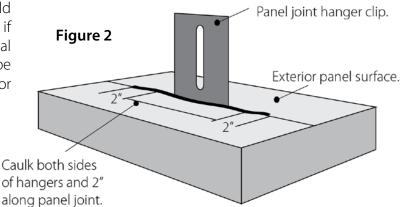
Note: Cut nozzle of caulking tube to a 45° for best results. Bead should be 3/16" wide.
